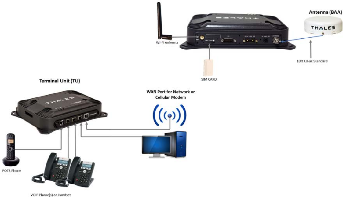
Figure 1-1 MissionLINK™ System with Connected Hardware
