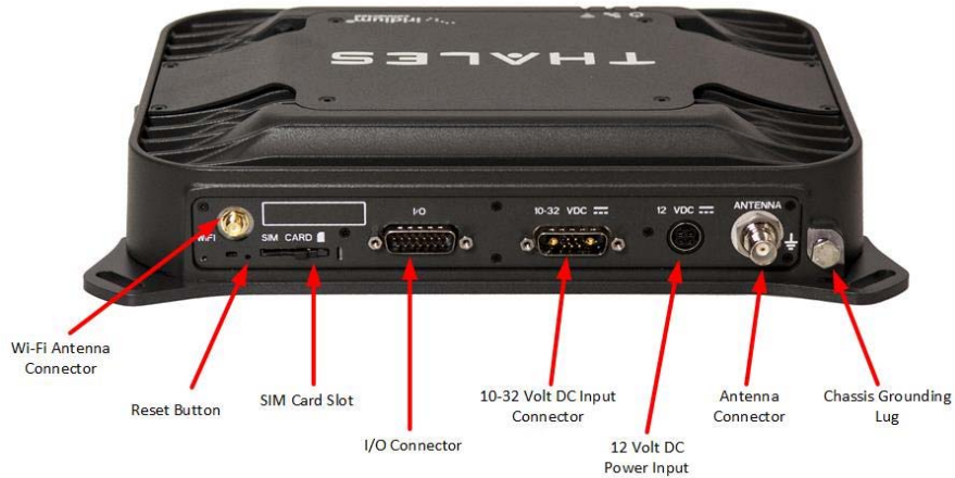
Figure 1-5 Terminal Unit (TU) Back Panel Detail
