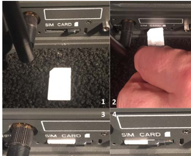
Figure 2-5 Installing SIM Card and Engaging the Lock
